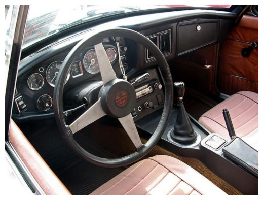
The MGB's dashboard was redesigned for the 1972 model year, restoring the glove box, and again in 1977 to meet revised U.S. safety regulations. This 1974 GT has new stalk-mounted controls for the lights and wipers, adopted on V8 cars the previous year.
