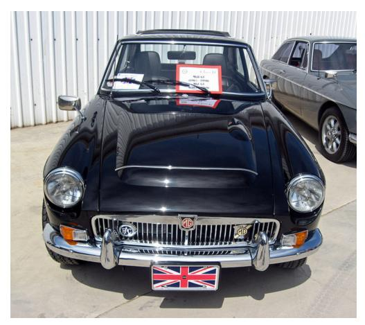
A rare North American MGC. The MGC's distinctive bonnet bulge (with a second, smaller bulge for the carburetors) was necessitated by the installation of the big C-series six, shared with the Austin 3-litre. The MGC was not a commercial success and only about 9,000 were built before production ended in August 1969.
