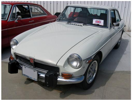
The 1974 MGB's rubber overriders — nicknamed "Sabrinas," after a particularly buxom British actress of the fifties — added about 6 inches (152 mm) to the B's overall length. North American models were now down to 78.5 horsepower (58 kW), thanks to a lower compression ratio and other changes for EPA emissions certification. This was the final year for the U.S. MGB GT; the hatchback coupe was withdrawn in early 1975, although it remained on sale in the UK.
