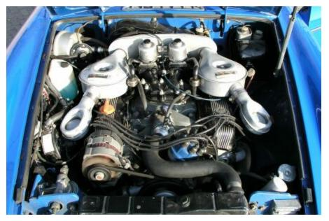
Although quite a few MGB owners have performed private engine swaps, this car has the factory V8's unusual "lobster claw" intake manifold, which enabled the Rover engine to fit in the B's engine bay without an MGC-style bonnet bulge. With two S.U. HIF6 carburetors, the 3,528 cc (215 cu. in.) engine was rated at 137 hp DIN (101 kW) and 193 lb-ft (261 N-m) of torque. (Photo © 2007 <u>Axel Volker</u>; used with permission)
