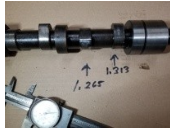
Figure 2: Used Damaged Camshaft
