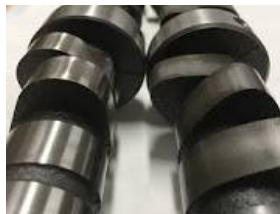
Roller on the left, flat tappet right
